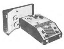
A self-contained, general-purpose, portable magnetic wire recorder and player. It comes complete—ready to use—with microphone and three spools of wire and connections for hookup to radios, public address systems, etc. It can be readily carried and takes up no more space than an overnight baq.
