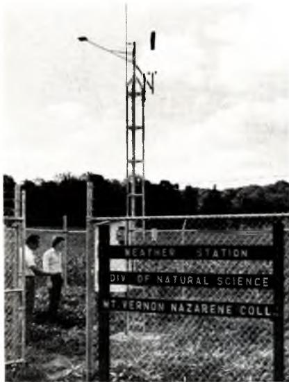
The Mount Vernon Nazarene College weather station, located 100 feet from the college's radio station tower, is in full operation. The automated station can monitor air temperature, relative humidity, soil temperature, soil moisture, wind direction, wind velocity, precipitation, solar radiation, and barometric pressure. The station was recently completed with a Title III grant.
